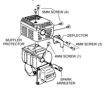
Figure 30. Spark Arrester Removal
